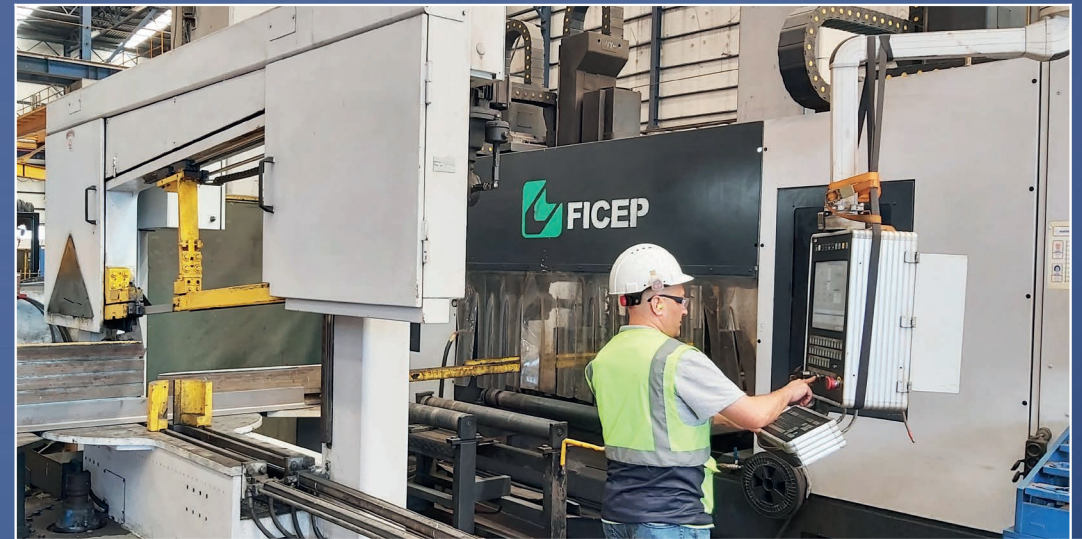
CNC PROFILE CUTTING - DRILLING
